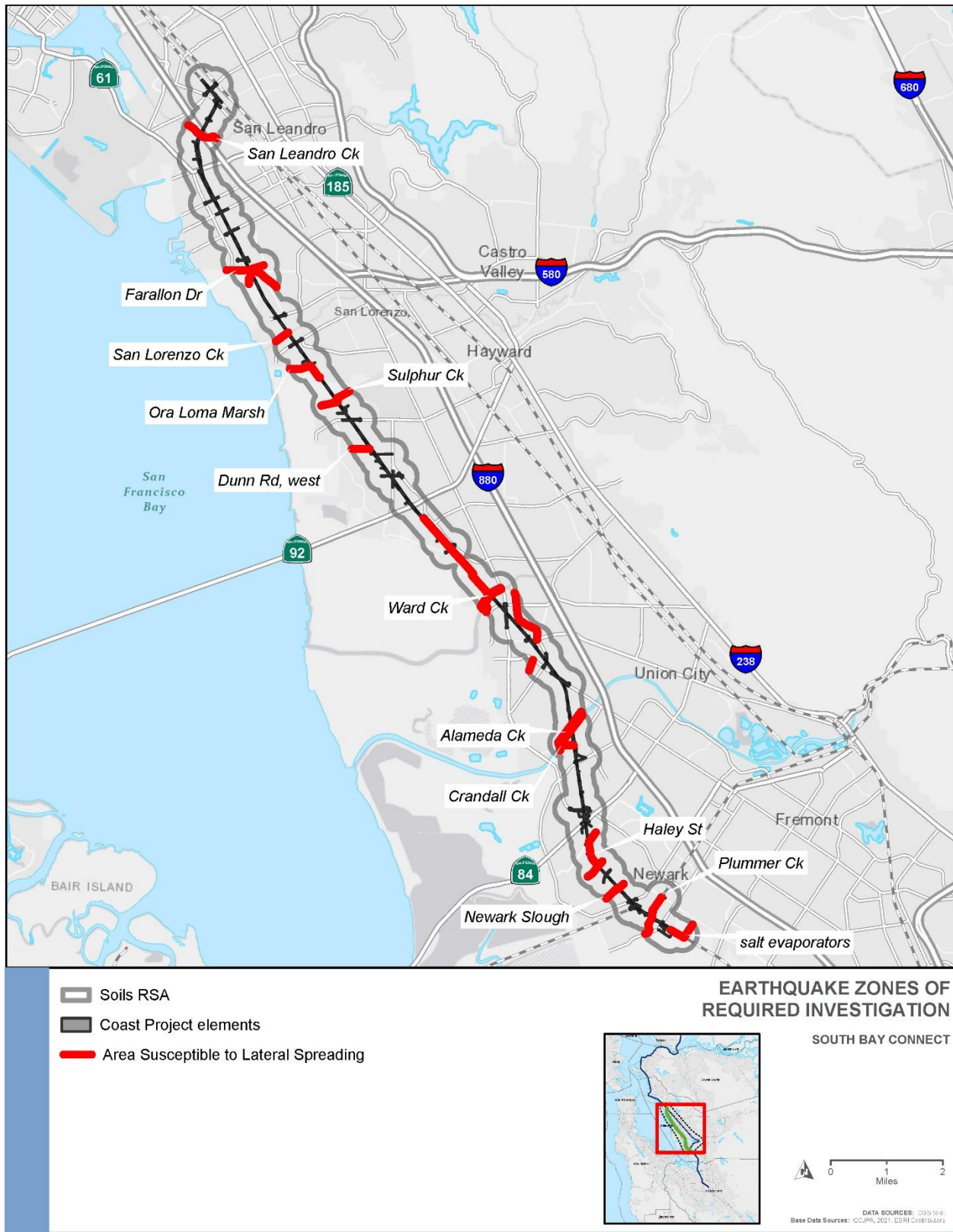
Figure 3.8-14: Locations Within the Geologic RSA With a Potential for Seismically Induced Lateral Spreading.
